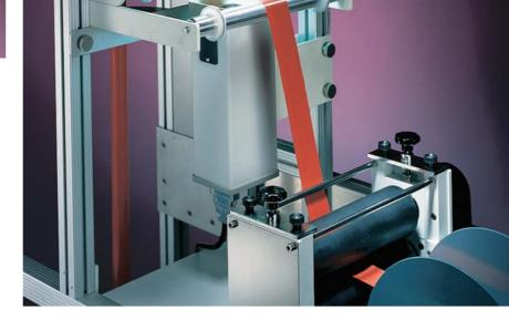
HAAKE PolyLab System: the comprehensive torque rheometer system for lab and pilot plant.
